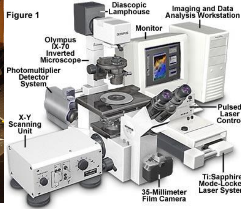
Multiphoton Excitation Fluorescence Microscope Configuration
